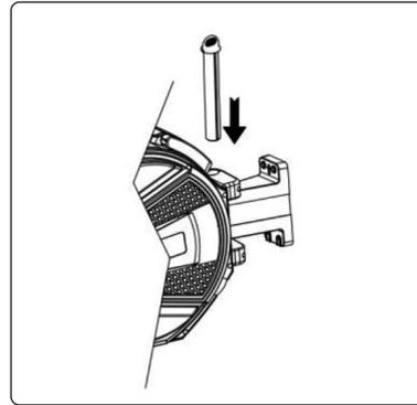
Align hose reel assembly with the holes in the bracket.
