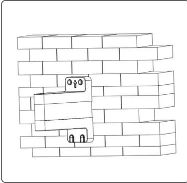
Use wall bracket to mark 4 x holes on a suitable wall or other secure structure.
